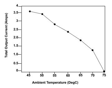
Thermal Shutdown Protection prevents damage to the device if temperature specifications are exceeded.
